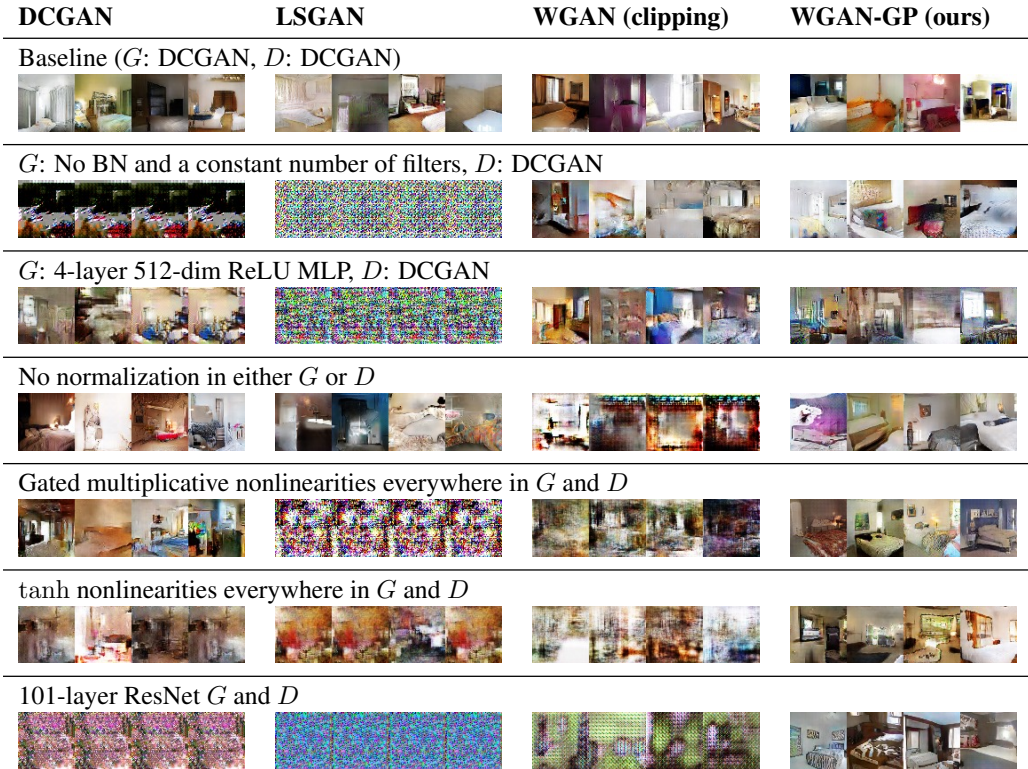
Figure 2: Different GAN architectures trained with different methods. We only succeeded in training every architecture with a shared set of hyperparameters using WGAN-GP.
