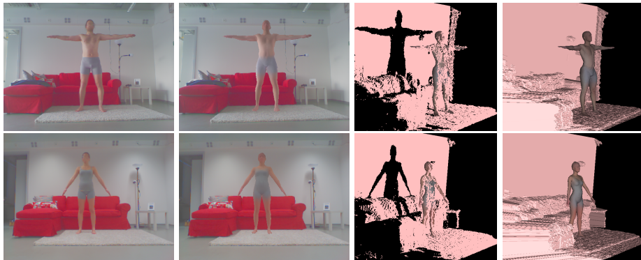
Fig. 9. Reconstruction of two subjects (top and bottom). First column: original captured images, with faces blurred for anonymity. Second column: simulated images after convergence. Third column: captured point cloud together with estimated body model. Fourth column: estimated body shown on background point cloud. More examples can be found in the supplemental materials.
