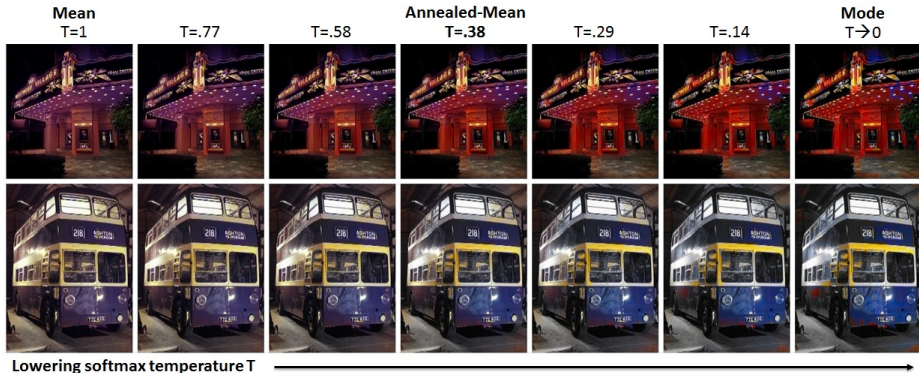
Fig. 4. The effect of temperature parameter T on the annealed-mean output (Equation 5). The left-most images show the means of the predicted color distributions and the right-most show the modes. We use T = 0.38 in our system.
