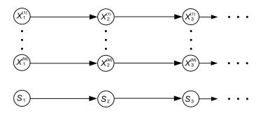
Figure 4: Graphical model representation for the structured variational approximation to the posterior distribution of the hidden states of a switching state-space model.
