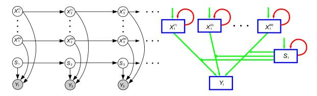
Figure 3: a) Graphical model representation for switching state-space models.  $S_t$  is the discrete switch variable and  $X_t^{(m)}$  are the real-valued state vectors. b) Switching state-space model depicted as a generalization of the mixture of experts. The light arrows correspond to the connections in a mixture of experts. In a switching state-space model, the states of the experts and of the gating network also depend on their previous states (dark arrows).
