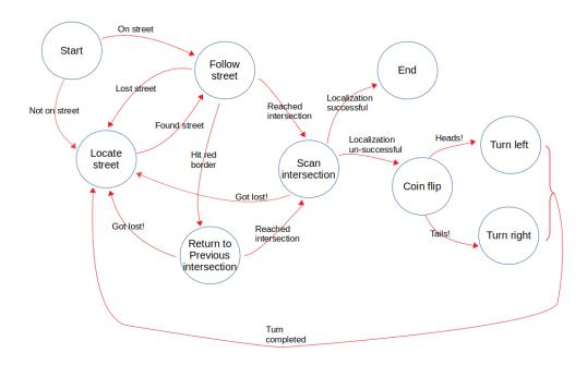
A few things are worth noting from the diagram. First, there is always a *start state* which takes care of any initialization required for the robot (in this case, setting up initial probabilities for each intersection, and figuring out if the robot is or is not on a street at the beginning of the process). There is also an *end state* which is reached once the robot has achieved its (or one of its) goal(s).
