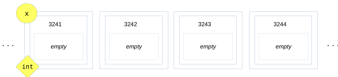
Figure 2.4: The same memory section from Fig. 2.3, after our program has requested space for an integer variable called x .
