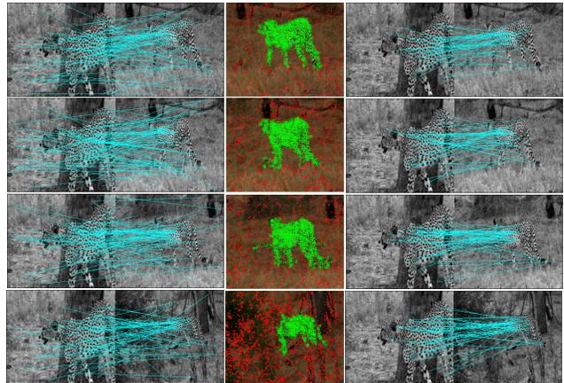
Figure 6. Tracking a cheetah against a complex background. **Left column:** Standard unconstrained matching between a video frame and the reference image that appears in the top-left corner of Fig. 1. **Middle column:** Foreground/background clusters produced by our method for the target video frame. **Right column:** Constrained matching results.
