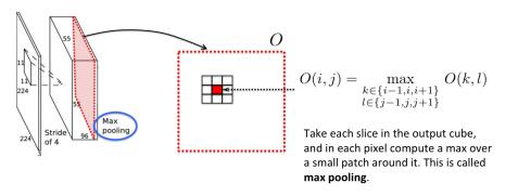
• Now add another "layer" of filters. For each filter again do convolution, but this time with the output cube of the previous layer.
