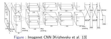
Complex mapping F(x, y, w) to predict output y given input x through a series of matrix multiplications, non-linearities and pooling operations
