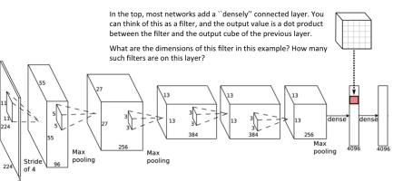
Add one final layer: a classification layer. Each dimension of this vector tells us the probability of the input image being of a certain class.
