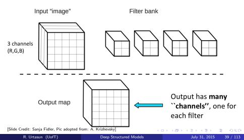
• So applying a filterbank to an image yields a cube-like output, a 3D matrix in which each slice is an output of convolution with one filter.
