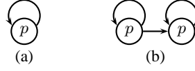
Fig. 1. Two models of a system in which p holds along every execution.
