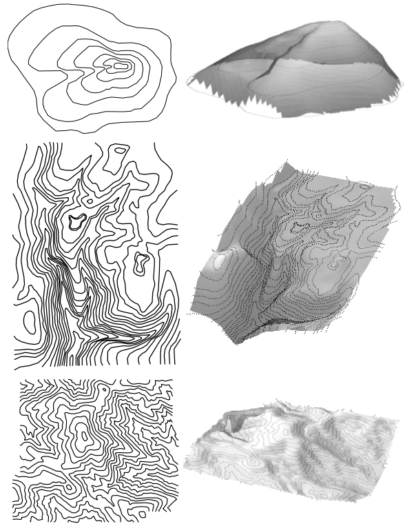
Figure 11. Reconstruction of topographic maps by piecewise planarity using a grid of 10 \times 10 cells. Each window is made of 2 \times 2 cells.
