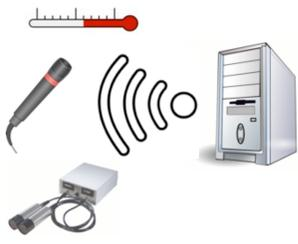
Information about the internal state of a physical device can be gained by making various measurements, such as temperature, sound, power consumption, and radiation.
