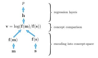
Fig. 2. Deep Learning architecture for regression, with three steps: encoding into concept-space, concept comparison and regression layers.
