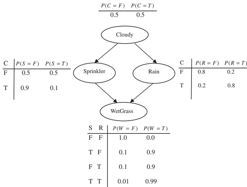
Fig. 2. This is an example of a multiply-connected BN, the original example graph can be found at Murphy (1998). The graph is redrawn for better quality.
