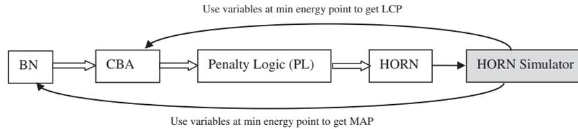
Fig. 1. An illustration for the framework we are proposing. First we convert the BN into an equivalent CBA system; then, we convert this CBA system into a strongly equivalent HORN. Through a HORN simulator, we can optimize the HORN energy function. HORN variables values at the minimum energy point will achieve both CBA LCP and BN MAP.
