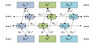
**Fig. 5.** Details of our bi-directional structure. The input of this structure is the features  $\{\mathbf{h}_i^0\}$  of multiple resolutions and contextual regions. Then bi-directional connections among these features are used for passing messages across resolutions/contexts. The output  $\mathbf{h}_i^3$  are updated features for different resolutions/contexts after message passing.
