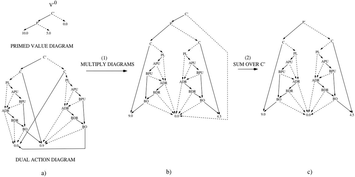
Figure 4: First Bellman backup for the *Value Iteration using ADDs* algorithm. (a)  $0$ -stage-to-go primed value diagram, and dual action diagram for variable  $C'$ ,  $Q_{C'}^a$ , (b) Intermediate result after multiplying  $V^{i0}$  with  $Q_{C'}^a$ . (c) Intermediate result after quantifying over  $C'$ .
