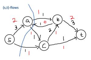
The red edge labels give an edge flow of 3 The blue cut allows a maximum of 3 across it from s to t Therefore 3 is optimal
