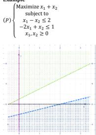
Let  $\hat{x} = \begin{bmatrix} 1 \\ 2 \end{bmatrix}$  and  $d = \begin{bmatrix} 1 \\ 1 \end{bmatrix}$ Then  $\hat{x} + \alpha d$  is feasible for all  $\alpha \ge 0$  and has objective value  $3 + 2\alpha$  so (*P*) is unbounded.
