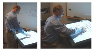
Figure 2. The touch table is oriented as a drafting table. Its height is set for both standing and sitting.
