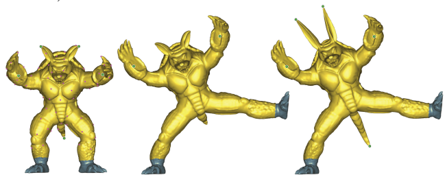
Figure 18: The user begins manipulating two points and two regions with the help of automatically positioned control points. Then the user adds handles interactively to stretch the ears and the tail.
