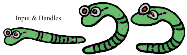
Figure 12: Auxiliary control points (purple) close to user-manipulated handles (green) are not a problem (middle figure). However, too close handles can lead to unpleasing deformations (right figure).
