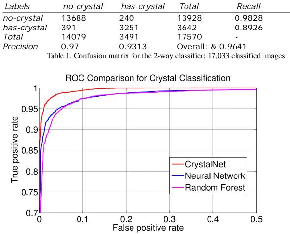
Fig. 3 ROC curve for bi-classification of crystal
