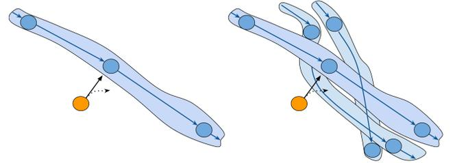
**Fig. 2: Examples of Trajectory Optimization in a Sparse and Dense Tree.** The blue tubes illustrate the domain covered by edges of the tree. The orange circle is a random state that we attempt to connect to its nearest state in the tree with trajectory optimization. The dotted curves are the trajectories followed when attempting the connection. The figures show that the attempt is more likely to be successful in a dense tree (right figure) than in a sparse tree (left figure).
