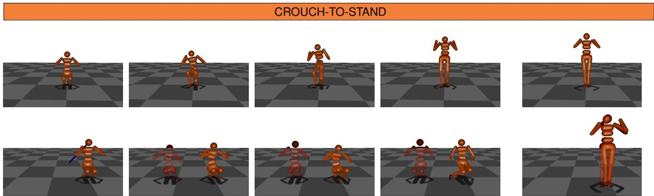
**Fig. 7: Crouch-to-Stand Controller.** The top sequence consists of key-frames of the crouch-to-stand controller. The bottom sequence illustrates how DOA expansion steers the character to the target (the state in the first frame of the top sequence). The blue line on the first frame is an external force applied on the head. The red character is the pose of the currently active node.
