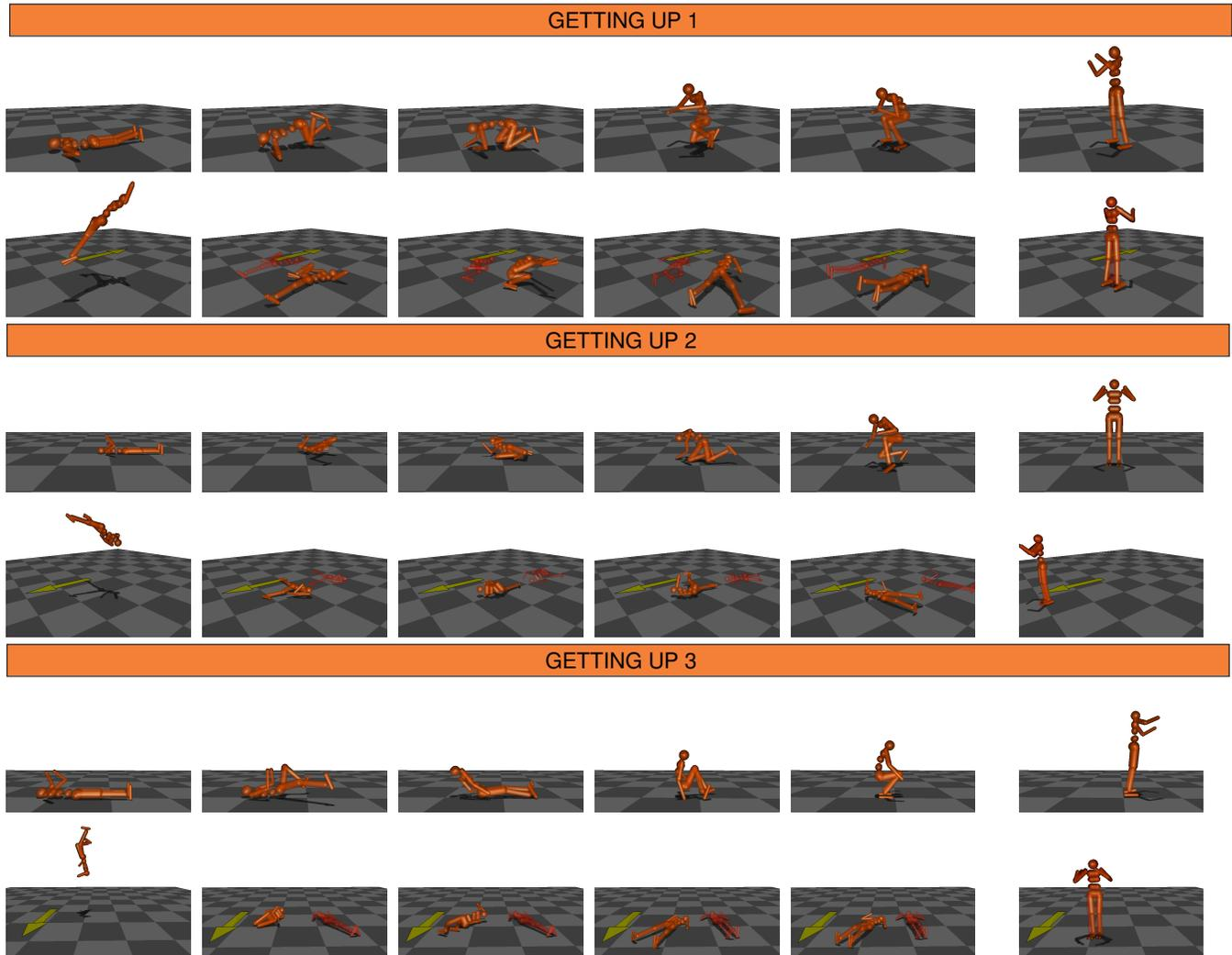
**Fig. 6: Getting Up Controllers.** The figure is divided into three pairs of sequences. For each pair, the top sequence illustrates an initial getting up controller and the bottom sequence illustrates how DOA expansion steers the character to the target (the state in the first frame of the top sequence). The yellow arrow points to the desired facing direction for the final pose of the character. The red character is the pose of the currently active node.
