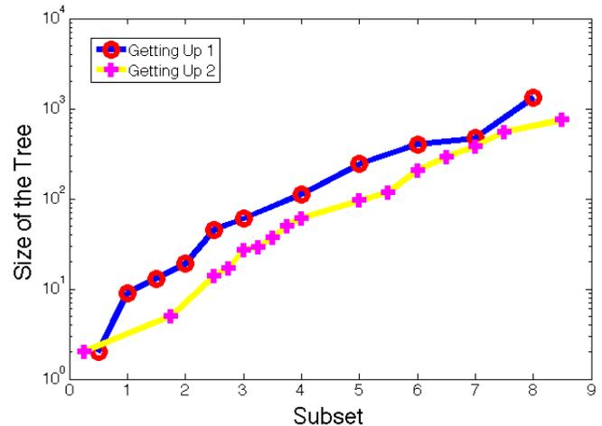
**Fig. 5: The Size of the Tree.** The figure plots the size of the tree in log scale required to cover a subset for the “Getting Up 1” and the “Getting Up 2” controllers. The subsets are parametrized by  $\alpha$ , which is defined in Sec. 4.3. In the plot, the value of  $\alpha$  is shown in the Subset-axis.
