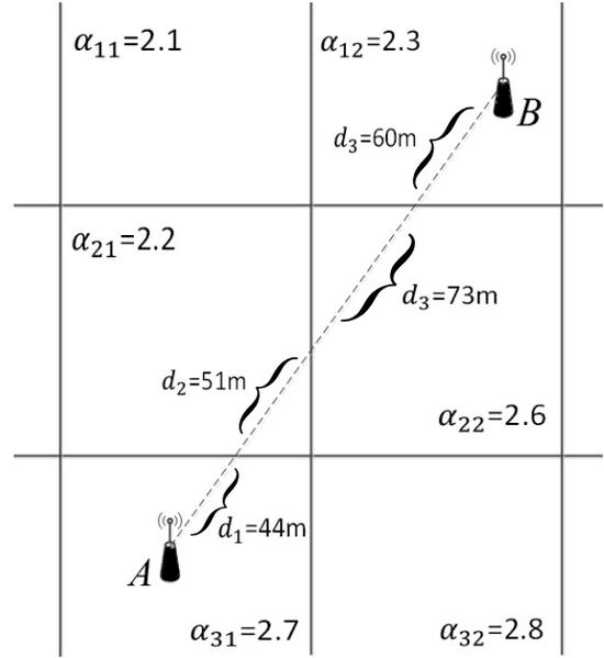
Fig. 2. Path loss example
