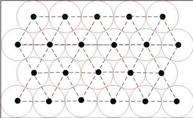
Fig. 6. Coverage is maximized at  $d = 2 \times S_r$ .
