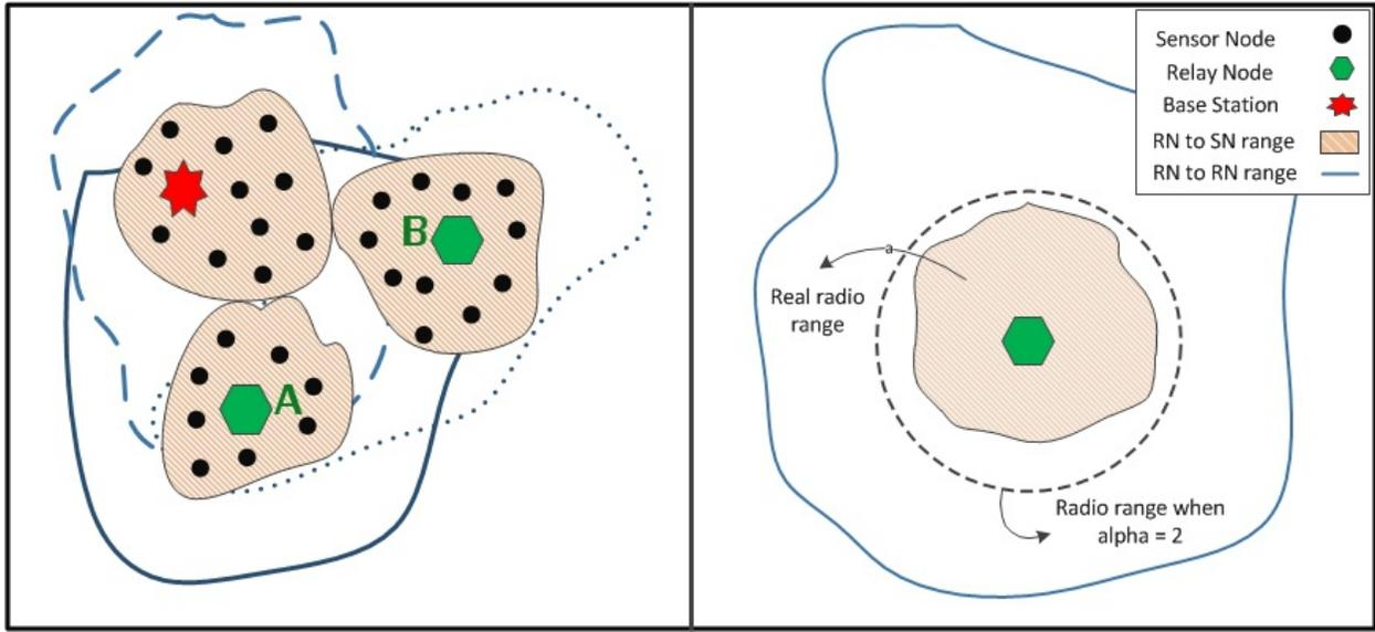
Fig. 3. Radio range in a real environment
