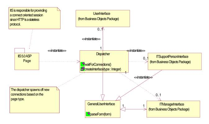
Figure 5 User Interface class diagram
