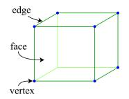
A polyhedron is a closed, connected polygonal mesh. Each edge must be shared by two faces.
