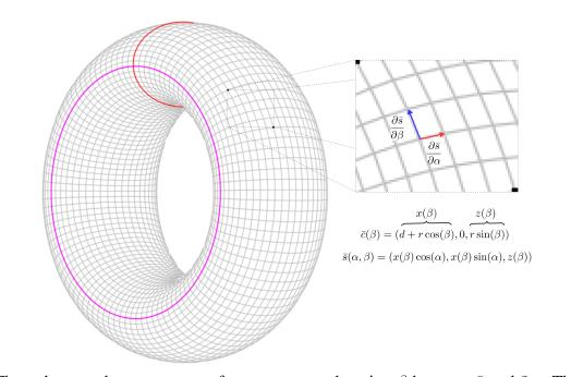
The red curve shows a contour for constant  $\alpha$ , changing  $\beta$  between 0 and  $2\pi$ . The purple curve shows a contour for constant  $\beta$ , varying  $\alpha$  between 0 and  $2\pi$ . The inset shows the two tangent vectors that form the tangent plane at a point on the surface.
