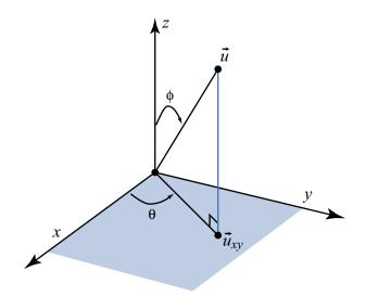
Given angles  $\phi$  and  $\theta$ , we can find a unit vector as  $\vec{u} = (\cos(\theta) \sin(\phi), \sin(\theta) \sin(\phi), \cos(\phi))$ .
