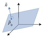
• Parametric:  $\bar{s}(\alpha,\beta) = \bar{p}_0 + \alpha \vec{a} + \beta \vec{b}$ , for  $\alpha,\beta \in \mathbb{R}$ .
