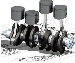
A 3D CAD model of an engine part. [Source: Wikipedia, author: Freeformer]
