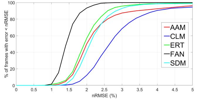
Fig. 2. Convergence curves for the pre-trained face alignment models, showing the nRMSE (%) vs. the percentage of frames with landmark localization error lower than the corresponding nRMSE threshold.
