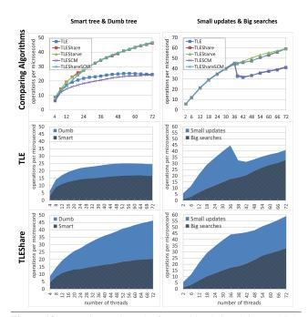
**Figure 13.** Experimental results for workloads involving multiple AVL trees. The top two graphs compare the performance of the TLE algorithms. The bottom four graphs each show a single TLE algorithm, and break out the performance of *each data structure*. The area graphs are *stacked*, meaning that the top of the upper area represents the aggregate performance for both trees.
