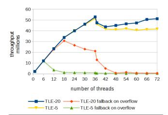
**Figure 2.** TLE using different retry policies on a large HTM system with 100% updates on an AVL tree with key range [0, 131072).
