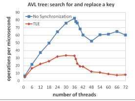
Figure 5. Comparison of TLE vs. no synchronization in a workload doing search-and-replace operations on an AVL tree with key range [0, 4096).
