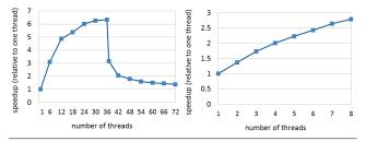
**Figure 1.** AVL tree microbenchmark on a large HTM system (left), and a small HTM system (right). The workload is 100% updates with key range [0, 2048).
