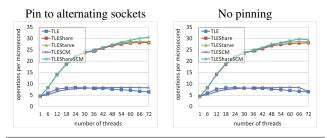
Figure 12. Experimental results for AVL trees with different thread pinning policies. The workload is 100% updates with key range [0, 2048).
