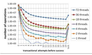
Figure 3. Histogram showing how many transactional attempts are made before a transaction successfully commits in a workload with 100% updates on an AVL tree with key range [0, 131072). After 20 attempts, the lock is taken. Note the log-scale.
