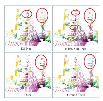
Figure 1: Comparison of our proposed method with DS-Net [15] and TORNADONet [11] on SemanticKITTI benchmark [1]. DS-Net and TORNADONet suffer from oversegmentation problem, while ours shows successful panoptic predictions.
