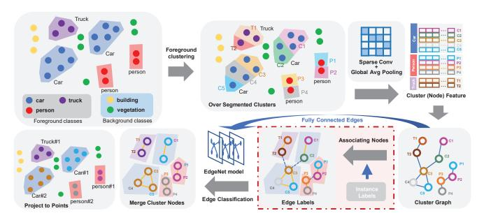
Figure 2: Illustration of GP-S3Net instance learning procedure. The input to the instance network is semantically segmented point cloud from the semantic network. The output is the list of instance clusters for foreground classes which will be fused with background classes to form panoptic results. Instance labels generation block drawn in red dashed box is ON only during training.
