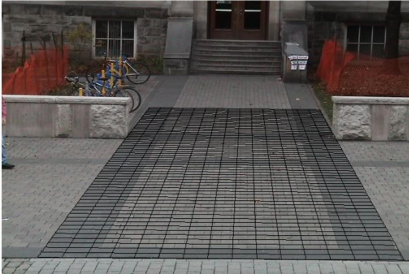
Camera calibrated with respect to ground plane.
