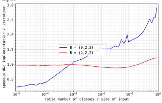
(d) *Histogram*: speedup of two divide-and-conquer implementations with respect to the input single-pass implementation, with varying ratio of number of input classes to total input size.
