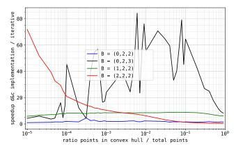
(f) *Quadrant orthogonal convex hull*: speedup of two divide-andconquer implementations with respect to the input single-pass implementation, with varying ratio of number of points in the convex hull to total input size.
