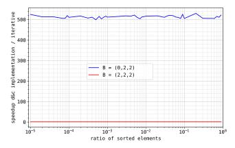
**(b)** *Closest pair*: speedup of two divide-and-conquer implementations with respect to the input single-pass implementation. PARSYNT synthesizes the solution with B = (0, 2, 2). The input is a sorted array of  $10^5$  elements, which are then swapped, and the y-axis represents the ratio of elements that are still sorted in the input.
