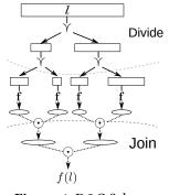
some extra information which **Figure 1.** D&C Schema is strictly required for  $\odot$  to recover f(l) from the partial computations of subtasks. **f** is a *lifting* (in the standard category theory sense) of f.
