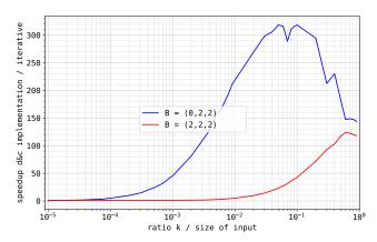
(a) *k*-largest: speedup of two divide-and-conquer implementations with respect to the input single-pass implementation, with increasing ratio of *k* to total input size. Input size is  $10^5$ . The synthesized solution for  $\mathcal{B}_{\odot} = (0, 2, 2)$  is compared to a naive quadratic solution (where the budget would be  $\mathcal{B}_{\odot} = (2, 2, 2)$ ).
