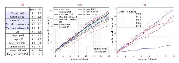
**Figure 7.** Splitting Divides: Table (a) lists the synthesis times (in seconds) of the benchmarks with splitting divides.  $\times$  indicates that the tool failed to find a solution. Figure (b) illustrates the speedups of the parallel implementations. Figure (c) compares the speedups of two parallel implementations of the LIS benchmark, for different ratios of size of increasing sequences to total size of input.
