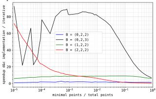
(e) *Minimal points*: speedup of three divide-and-conquer implementations with respect to the input single-pass implementation, with varying ratio of number of minimal points in input to total input size.
