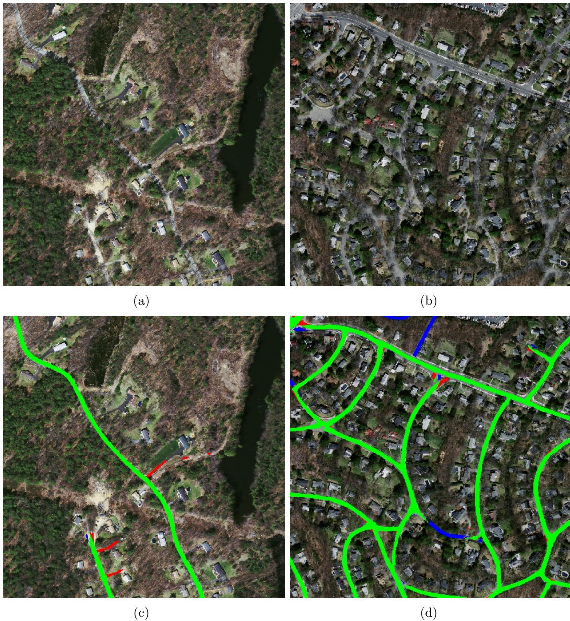
Figure 6.2: Figures 6.2(a) and 6.2(b) show two representative regions from the Massachusetts Roads dataset. Figures 6.2(c) and 6.2(d) show predictions of a post-processing network on these regions.
