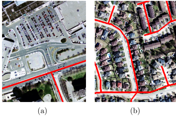
Figure 4.1: Road locations derived from a map are shown in red. (a) Example of omission noise. (b) Example of registration noise.
