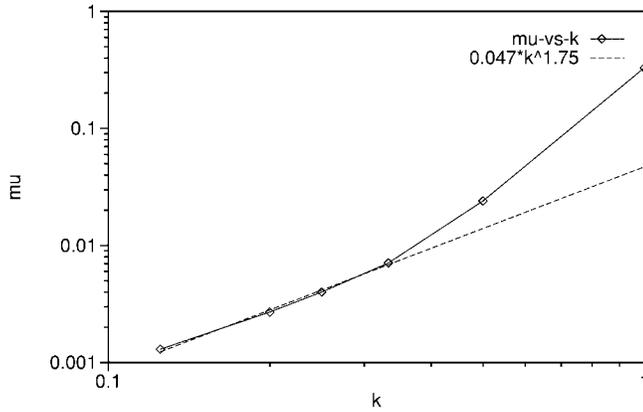
FIG. 5.—For  $k = 1, \frac{1}{2}, \frac{1}{3}, \frac{1}{4}, \frac{1}{5},$  and  $\frac{1}{8}$  and  $\epsilon \geq \frac{1}{4}N^{-1/3}$  of Fig. 4, the values of  $\mu_k$  were fitted by eye and are, respectively,  $\mu = 0.33, 0.024, 0.0071, 0.0040, 0.0027,$  and  $0.0013$ . These are plotted and, for  $k \leq \frac{1}{3}$ , fit the curve  $\mu = (0.047 \pm 0.015)k^{1.75 \pm 0.25}$ .
