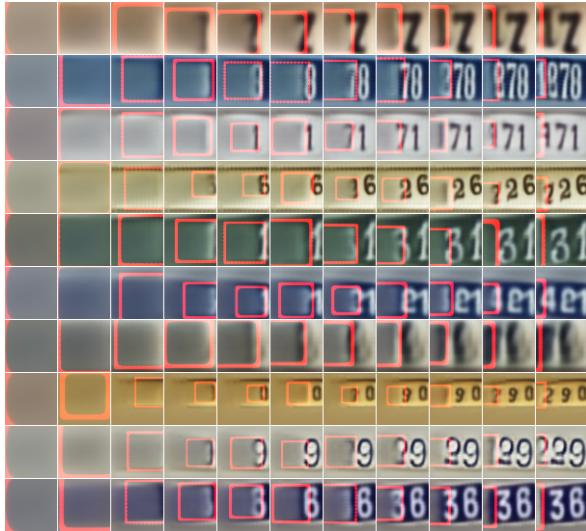
Figure 10. SVHN Generation Sequences. The red rectangle indicates the attention patch. Notice how the network draws the digits one at a time, and how it moves and scales the writing patch to produce numbers with different slopes and sizes.
