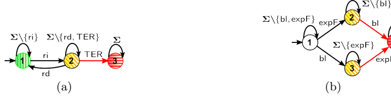
Figure 3: Monitors: (a) A_1 , (b) A_2 . Red states are shaded horizontally, green states are shaded vertically, and yellow states are shaded diagonally.
