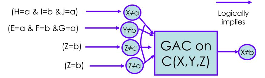
An immediate and computationally inexpensive clause we can obtain is simply the set of pruned values that caused the new pruning.
