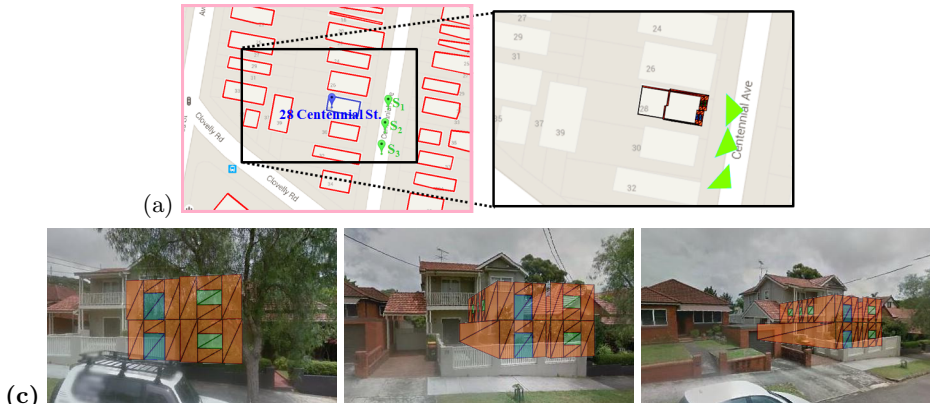
Fig. 2: The initial building’s position and StreetView images. In (a), blue pin shows the geo-reference result, green pins show three nearby StreetView images S_{1,2,3} , red lines depict the building contours parsed from the map image. (b): Building’s floor-plan placed on the map. (c) shows StreetView images corresponding to S_{1,2,3} in (a), respectively, overlaid with the virtual house rendered with the initial building position (from (b)) and floor, door, window heights as 1m, 2m, 3m.
