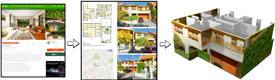
Fig. 1: We exploit rental ads and a small set of (wide-baseline) Google’s StreetView images to build realistic textured 3D models of the buildings’ exterior. In particular, our method creates models by using only the (approximate) address and a floorplan extracted from the rental ad, in addition to StreetView.
