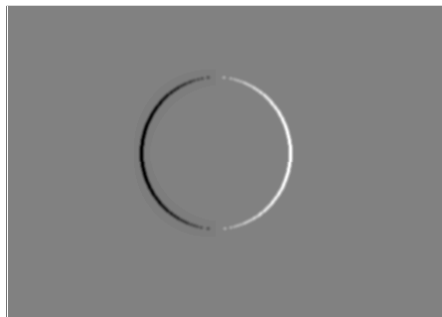
\frac{\partial f(x,y)}{\partial x} with [-1, 1] and correlation
