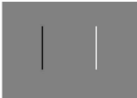
\frac{\partial f(x,y)}{\partial x} with [-1, 1] and correlation
