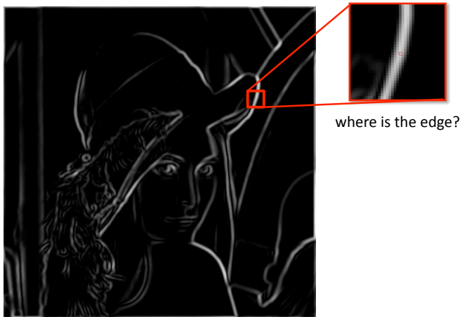
Figure: Gradient magnitude
