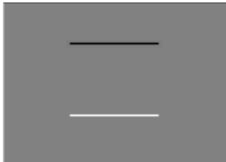
\frac{\partial f(x,y)}{\partial y} with [-1, 1]^T and correlation
