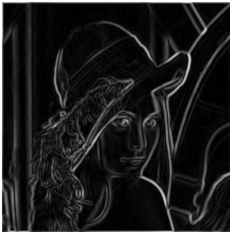
Figure: Canny's approach takes gradient magnitude
