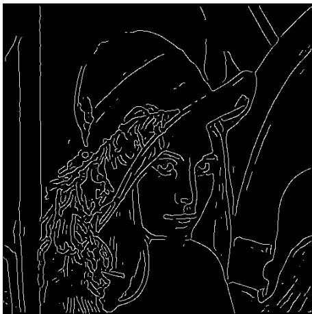
Figure: Thinning: Non-maxima suppression
