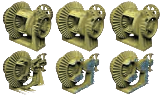
Fig. 9. Voxel stuffing produces a tetrahedral mesh (middle) of quality comparable to a direct BSP-tree construction (right), but reduces the running times from 3292.3 seconds to 2476.6 seconds.
