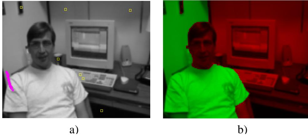
Figure 3.2: Effect of seed crossing an image boundary, a) source region (magenta) and sink pixels (yellow), notice that the source spills across two separate regions. b) min-cut result, under-segmentation occurs. The original image is  $160 \times 120$  pixels.
