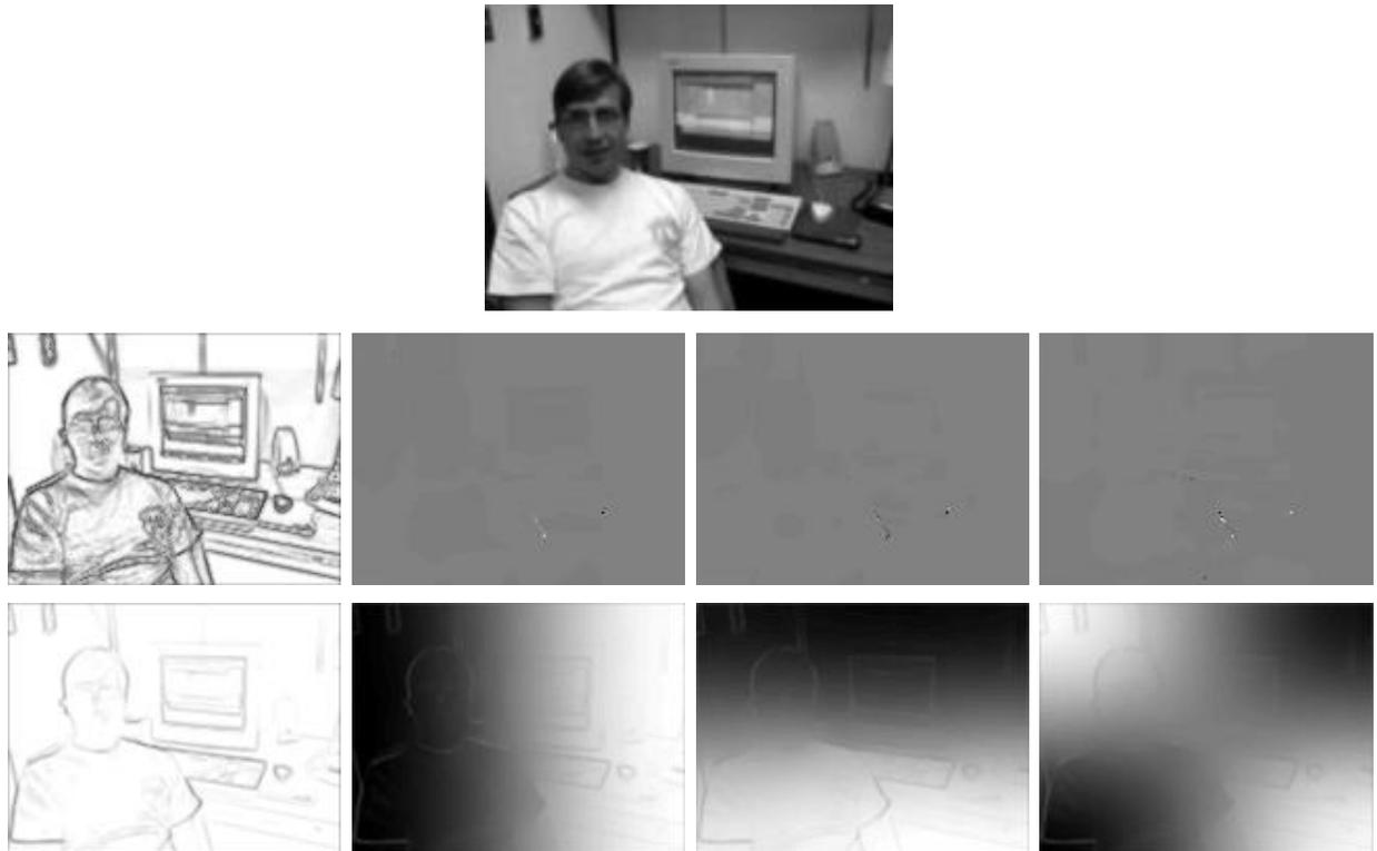
Figure 3.4: Top: Original image. Middle: Leading eigenvectors for  $\sigma = 4$ , with such a small  $\sigma$  the eigenvectors capture local perturbations created by a few pixels. Bottom: Leading eigenvectors for  $\sigma = 25$ . In this case  $\sigma$  is too large, and the eigenvectors are smoothed out. For such a large  $\sigma$  the eigenvectors resemble sinusoid functions.
