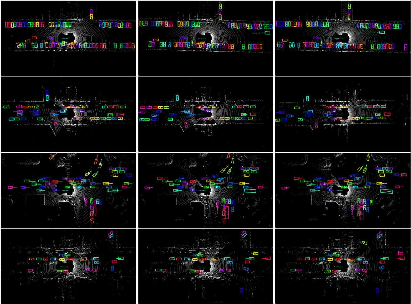
Figure 10: **Qualitative results on 144x80M region [best view in color]**. Same color represents same vehicle across different timeframe. Each vehicle has ‘dot’ presents the center locations of current and future time frames
